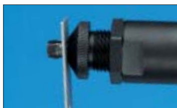
Insert the punch (fixed onto the 74290 tool) into the round hole
